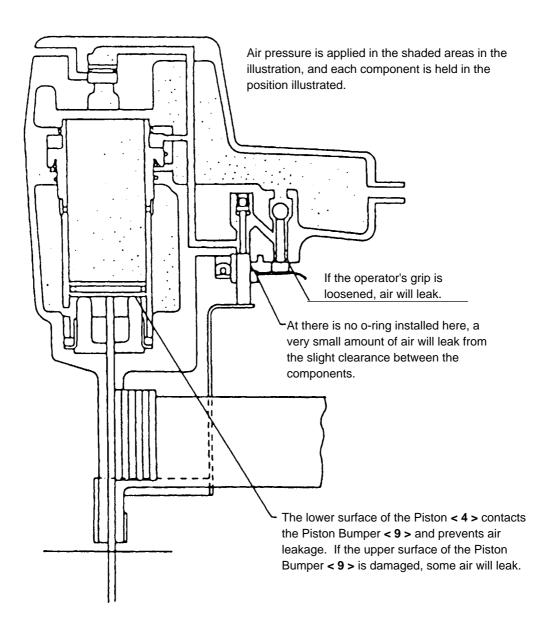
Fig. 7 If the trigger and pushing lever are kept pressed
