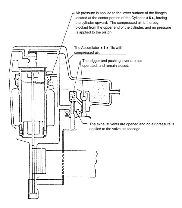
Fig. 5 When the compressed air source (air hose) is connected to the nailer
