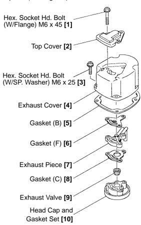
Fig. 13 Disassembly of main body, upper part
