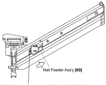
Insert a bar such as a screwdriver into this hole.
