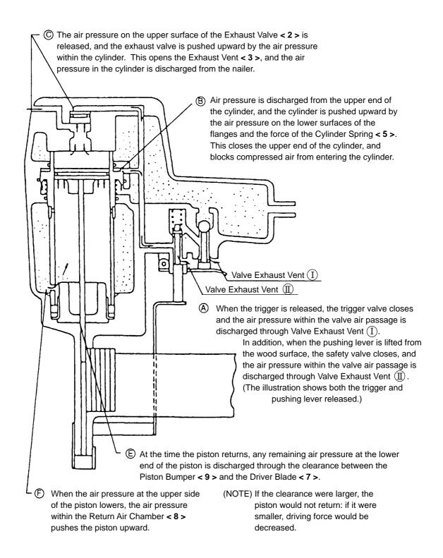
Fig. 8 When the trigger and/or pushing lever are released
