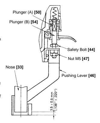
Fig. 17 Pushing lever adjustment
