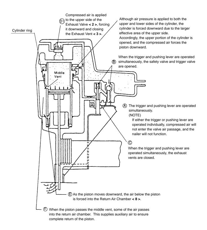
Fig. 6 When the trigger and pushing lever are operated
