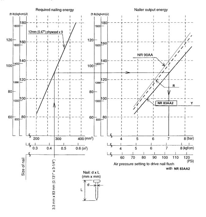
Fig. 2 Required nailing energy and nailer output energy
