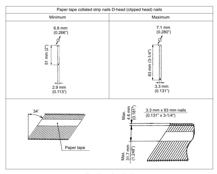
Fig. 1 Dimensions of nail
